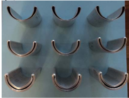
Figure 12. Test Samples ( D/t : 16.2, 23.8 and 47.6) after the CRST
