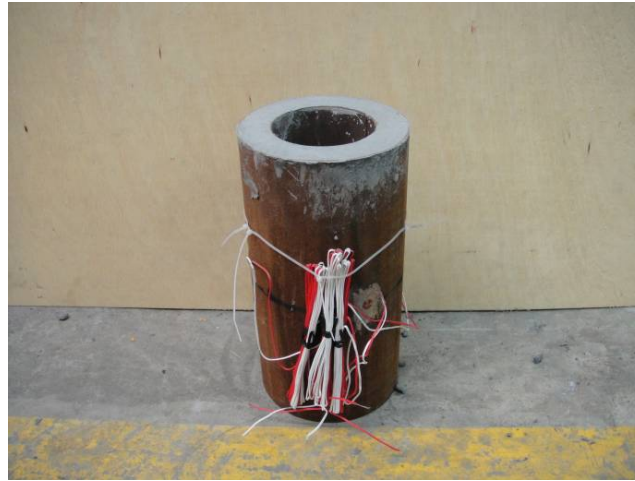
Figure 1(h) Double-skinned HSCFST columns without external steel ring with hollow ratio of 0.72
