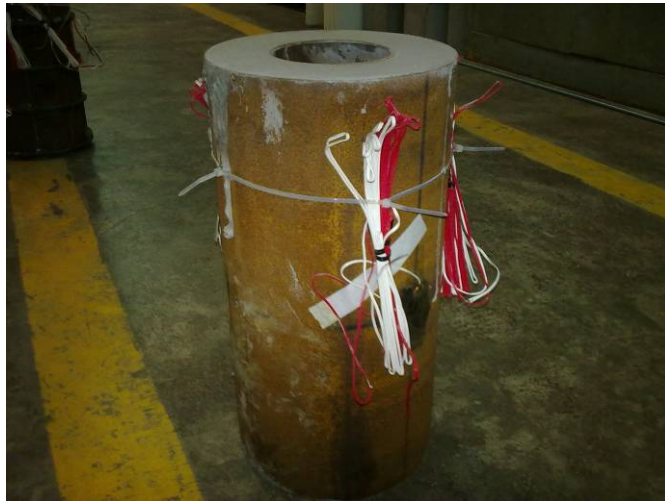
Figure 1(c) Double-skinned NSCFST columns without external steel ring with hollow ratio of 0.56
