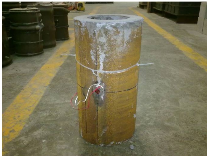
Figure 1(d) Double-skinned NSCFST columns without external steel ring with hollow ratio of 0.72
