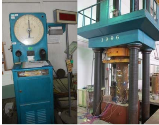
Figure 12. 1500T Hydraulic Pressure Testing Machine
