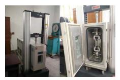
(a) The Tensile Testing Machine
