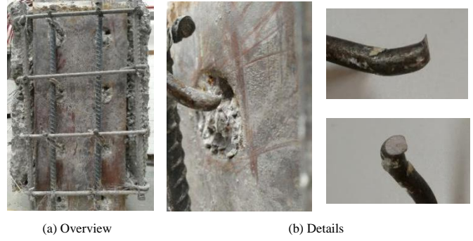
Fig. 13 Failure states of the perforated steel reinforcements and concrete in the holes
