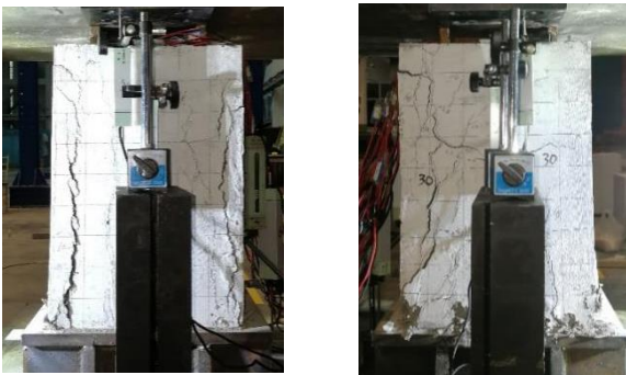
Fig. 12 The failure mode of PSSCC
