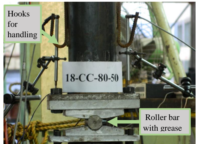
Fig 8 Arrangement of pinned boundary condition
