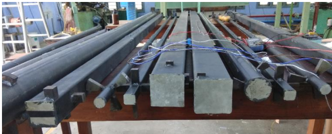
Fig. 5 Inner steel tubes with spacer bars and dummied concreting end
