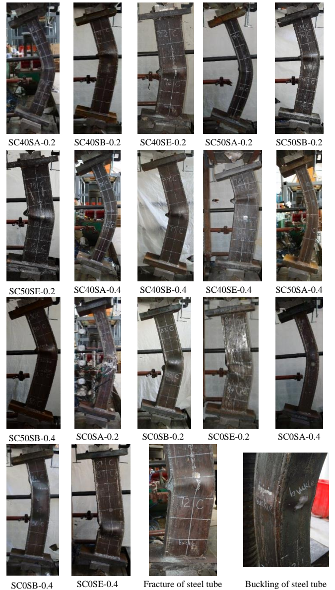
Fig. 5 Failure of the specimens
