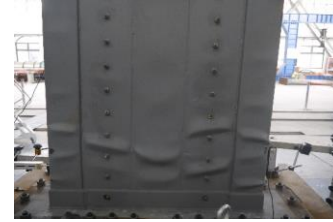
(e) Failure condition of GHQ-6 from the back view
