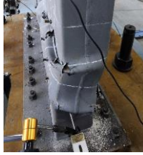
(a) Fracture propagation of steel and crushing of concrete in GHQ-1 (b) Failure condition of GHQ-3
