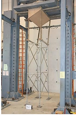
Fig. 19 Deformation of the combined system of scaffolds with wooden shores under inclined slab after loading ( \alpha=1.0/\theta=30^\circ in the in-plane direction)
