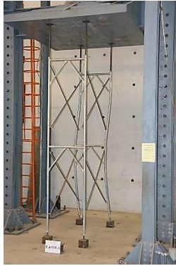
Fig. 11 Deformation of the scaffolding system with extended adjustable U-head jacks after loading
