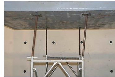
Fig. 14 Deformation of the adjustable U-head jacks of the scaffolding system with both extended adjustable U-head jacks and base jacks after loading
