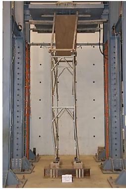
Fig. 26 Deformation of the combined system of scaffolds with wooden shores under inclined slab and uneven base after loading ( \alpha=0.7/\beta=0.15/\theta=30^\circ in the out-of-plane direction)
