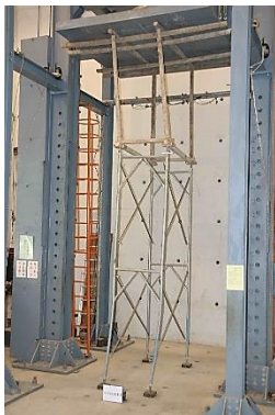
Fig. 16 Deformation of the combined system of scaffolds with wooden shores ( \alpha=1 ) after loading
