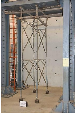
Fig. 18 Deformation of the combined system of scaffolds with wooden shores ( \alpha=0.382 ) after loading
