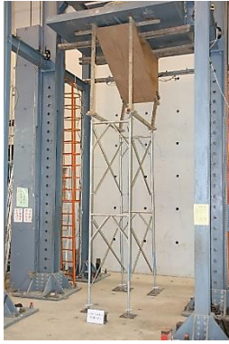
Fig. 22 Deformation of the combined system of scaffolds with wooden shores under inclined slab after loading ( \alpha=1.0/\theta=30^\circ in the out-of-plane direction)
