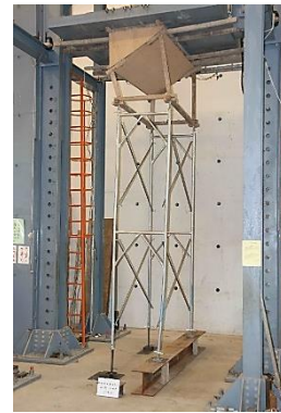
Fig. 25 Deformation of the combined system of scaffolds with wooden shores under inclined slab and uneven base after loading ( \alpha=0.5/\beta=0.15/\theta=30^\circ in the in-plane direction)
