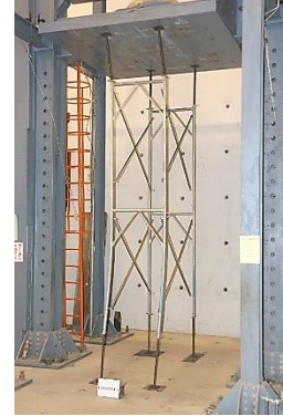
Fig. 13 Deformation of the scaffolding system with both extended adjustable U-head jacks and base jacks after loading
