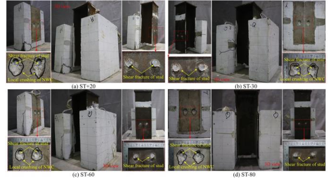
Fig. 13 Failure modes of push-out specimens of headed studs at low temperatures
