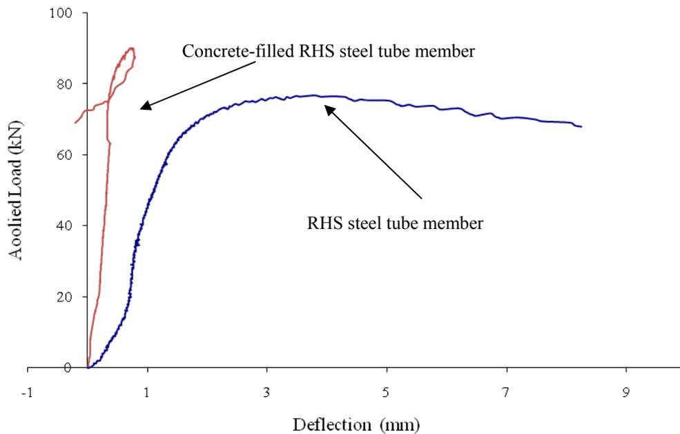
Figure 6. Load against Out-of-plane Deflection of Failure Member
