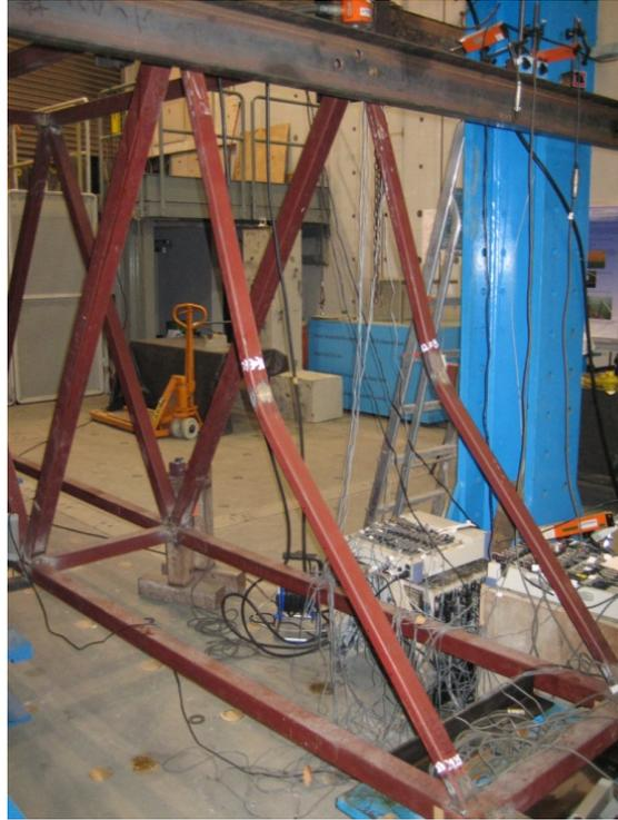
Figure 5. The Failure Shape of Composite Member Truss
