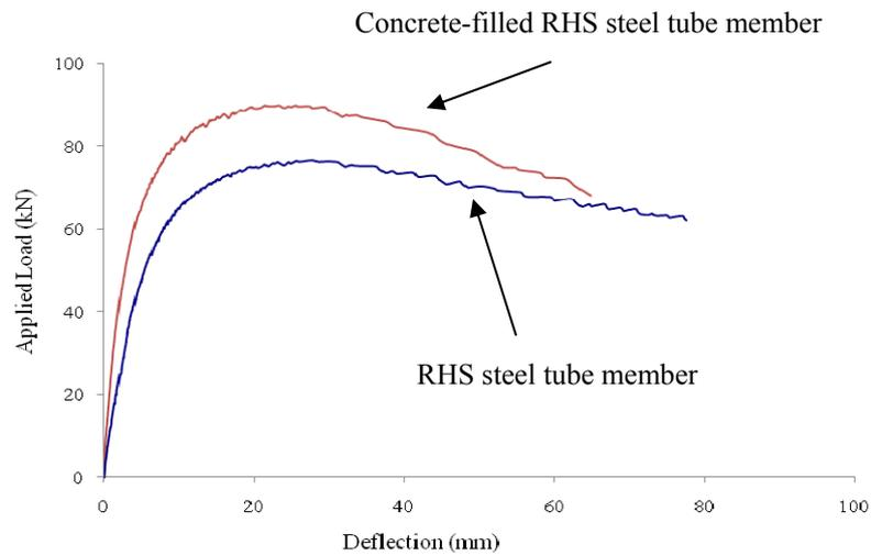
Figure 3. Load against in-plane Deflection of Failure Member
