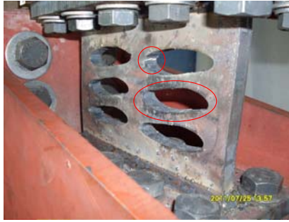
Failure of the damper studs of specimen 15Y
