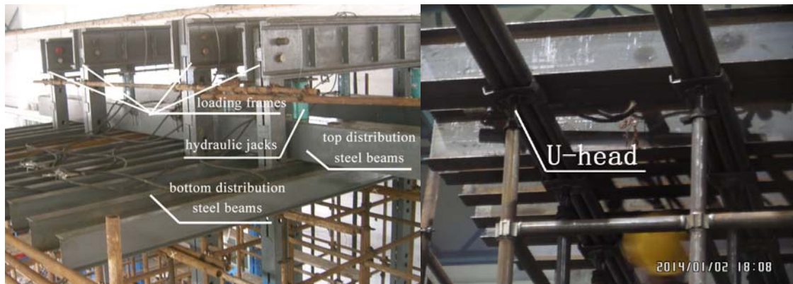
Figure 15. Loading Mechanism and Test Set-up
