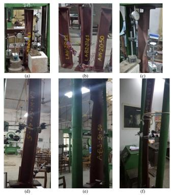
Fig. 9 Failure of specimens with different slenderness ratio and connections
