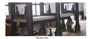
Fig. 1 Experimental setup for vertical cyclic load
