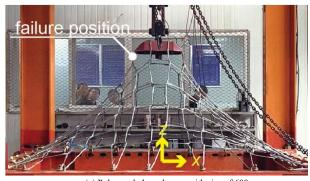
(e) Polygonal-shaped press with size of 600mm
