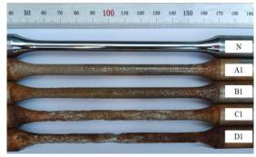
Fig. 5 Macro corrosion morphology of the specimens
