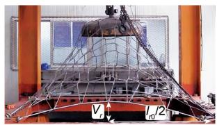
(a) Deformation of the wire rope
