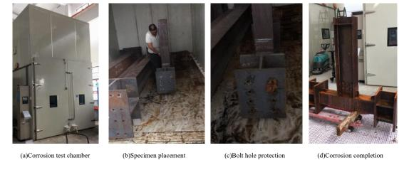
Fig. 4 Corrosion process of the specimen LZ-2
