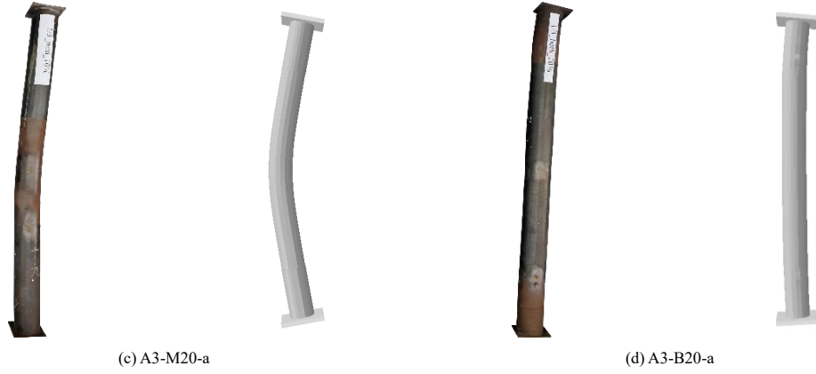
Fig. 4 Comparison of failure modes between test and finite element model
