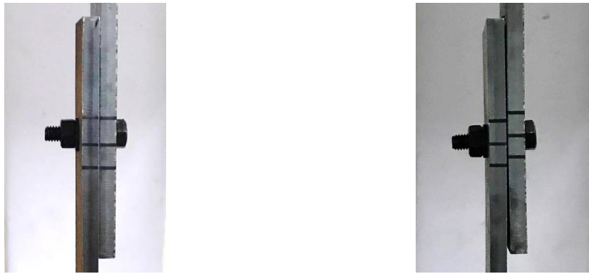
Fig. 13 Failure of bolt connection after testing
