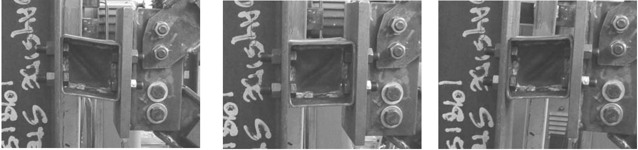
Figure 4.22. 1 mm single plate device during 20 mm cycles – from left to right: end of upward stroke; device brought back to zero deformation; end of downward stroke
