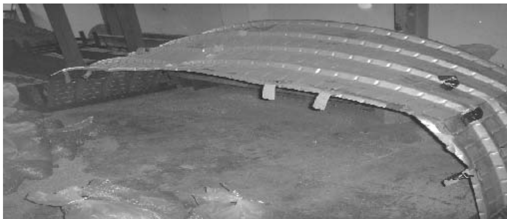
Figure 36. Experimental deflected shape of 1.0 m crown height parabolic roofing element
