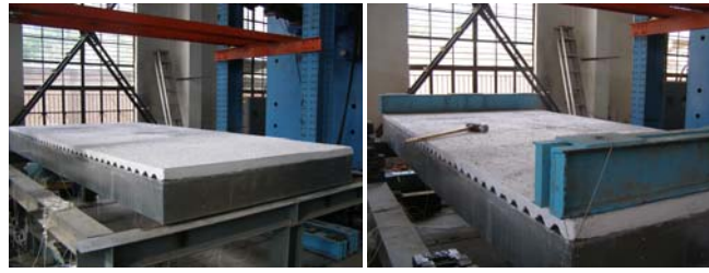
Figure 5. Constraint Condition Setup: (a) Simple Support Boundary; (b) Fixed Support Boundary
