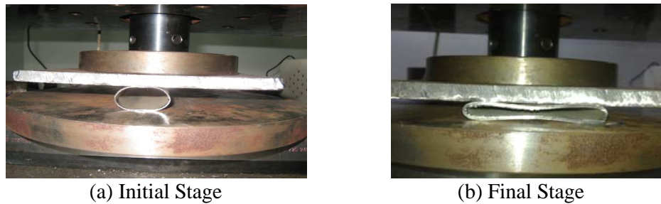
Figure 6. Static Compression Experiment of Single Circular Steel Tube
