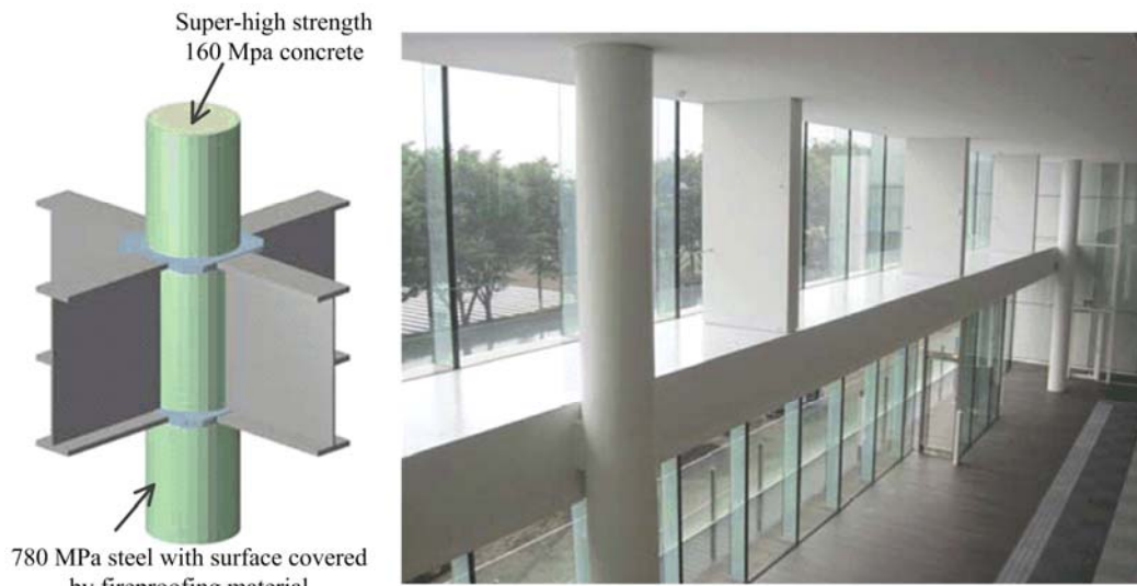
Figure 5. Application of 780 MPa High Strength Steel (adapted from [31])
