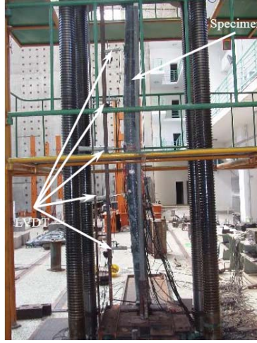
Figure 3. Test Arrangement (Specimen CC H-1)
