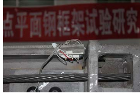
b) The gap opening width of the connection on the west side: 11.79 mm; gap opening rotation: 2.72%
