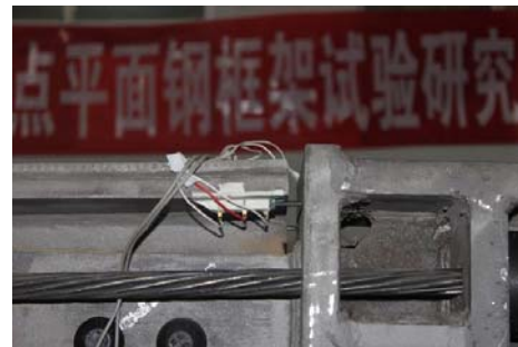
b) The gap opening width of the connection on the west side: 14.28mm; gap opening rotation: 3.29%
