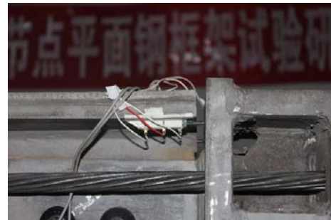
b) The gap opening width of the connection on the west side: 4.52 mm; gap opening rotation: 1.04%
