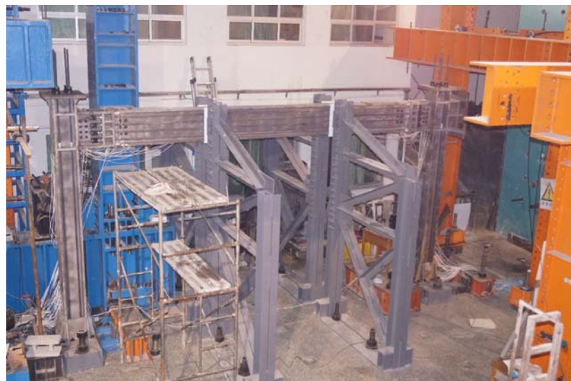
Figure 5. Photograph of the Loading Device used during the Test
