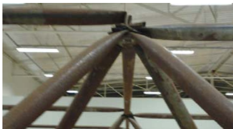
Figure 40. Collapse in Typical Model (24kN)
