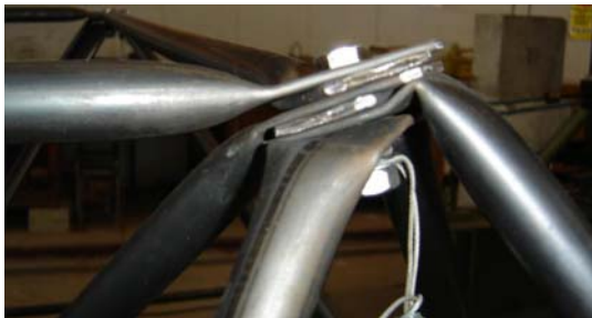
Figure 21. Collapse of the Typical Model (P2 - 25kN)
