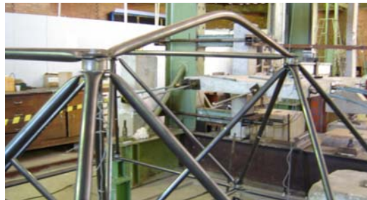
Figure 22. Collapse of Modified Model (P1 - 42kN)
