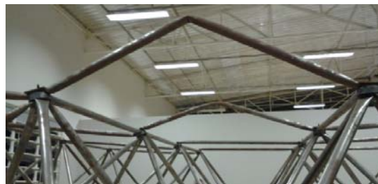
Figure 41. Collapse in Modified Model (35.1kN)
