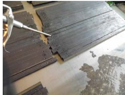
(b) Gauge hole cleaning
