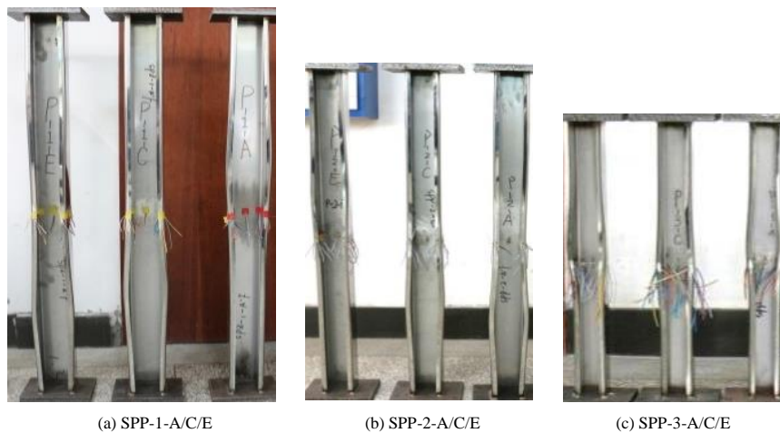
Fig. 15 Failure of positive eccentrically loaded specimens
