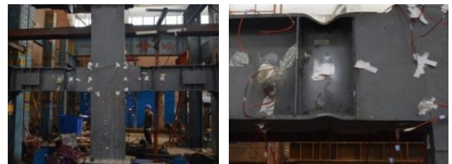
(a) Final failure state (b) Buckling of flange
