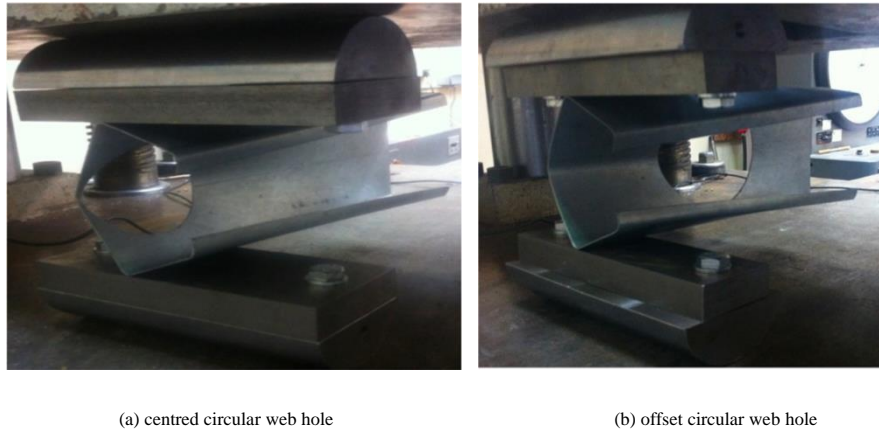
Fig. 3 Experimental analysis of lipped CFS C-sections (unfastened flanges) under ETF loading condition from Uzzaman et al. [26]
