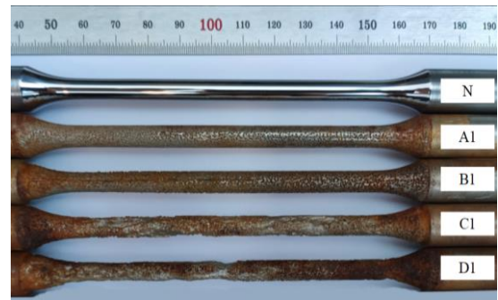
Fig. 5 Macro corrosion morphology of the specimens
