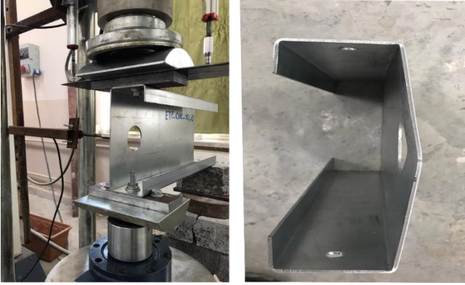
Fig. 10 ETF_CIRC_50_0 specimen test setup and failure mode
