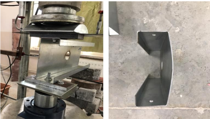
Fig. 12 ETF_CIRC_50_150 specimen test setup and failure mode
