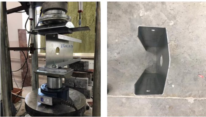
Fig. 11 ETF_CIRC_50_50 specimen test setup and failure mode
