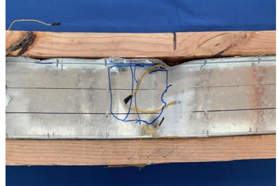
(b) Buckling of the profile flange observed in the L-6 beam compression zone
