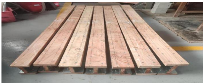
Fig. 2 Finished steel-wood combination beam member
