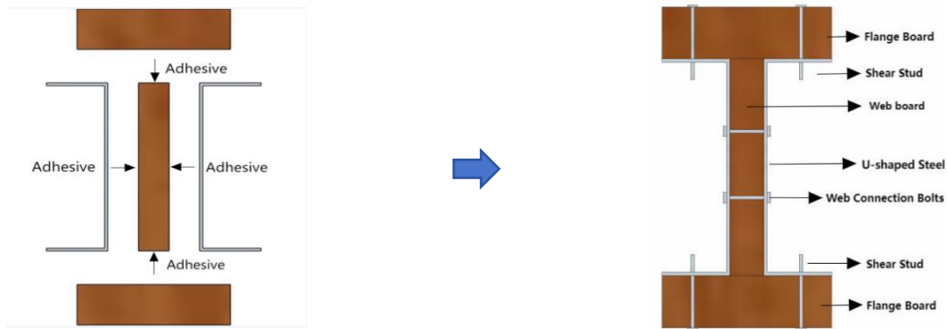
(a) Cross-section of steel-wood combination beam
