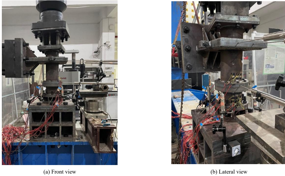
Fig. 7 Test setup for a connection joint
