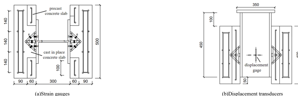
Fig. 4 Arrangement of strain gauges and displacement meters
