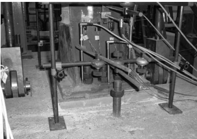
Figure 3. Close-up of the electrical displacement transducers (LVDTs): traditional ( left ) and innovative ( right ) joint.
