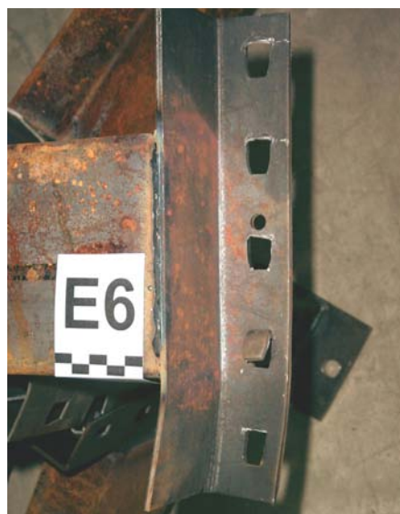
Figure 16. Deformation of Connector Observed during the Tests
