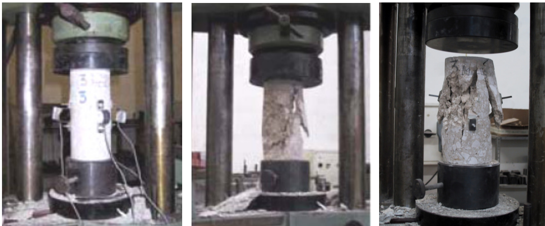
Figure 9. Compression Test on Concrete Cylindrical Specimen
