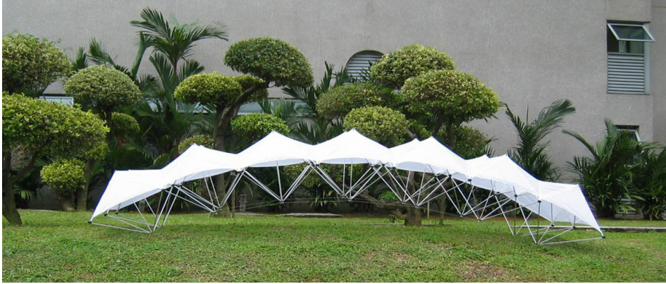
Figure 7. Ultra-lightweight Scale Model of Umbrella DSMTS
