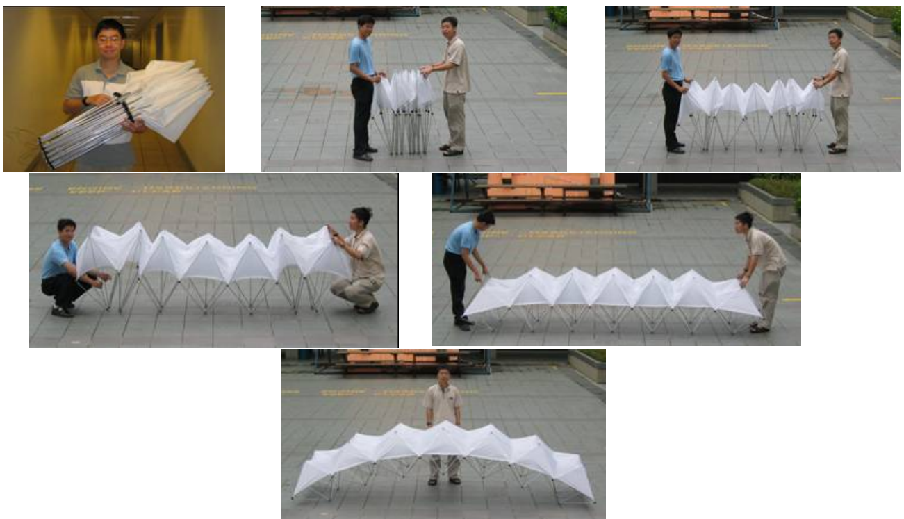
Figure 8. Deployment Process of Umbrella DSMTS Prototype
