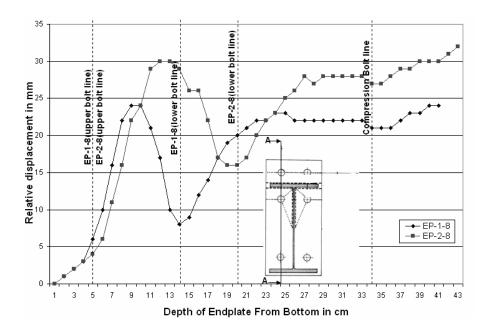
Figure 9. Endplate Relative Displacements of 8mm Thick Endplates
