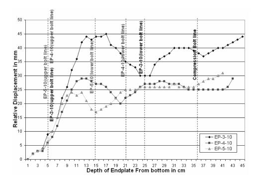
Figure 10. Relative Displacement of 10mm Thick Endplates
