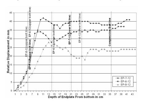
Figure 11. Relative Displacement of 12mm Thick Endplates
