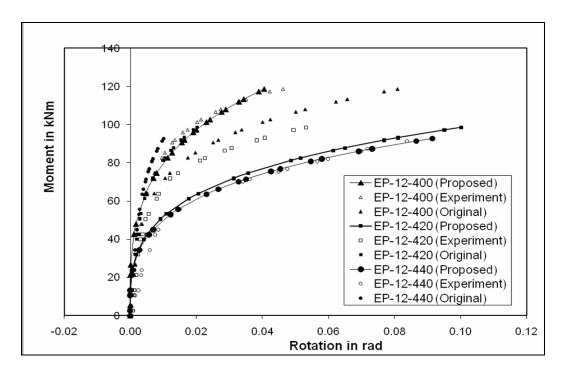
Figure 21. Comparison of M- $\theta_r$  Curves of Proposed Model with Experiment and Original Model for All 12 mm Specimens
