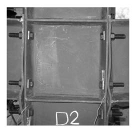
Figure 5. Contact Opening of Endplate Connection
