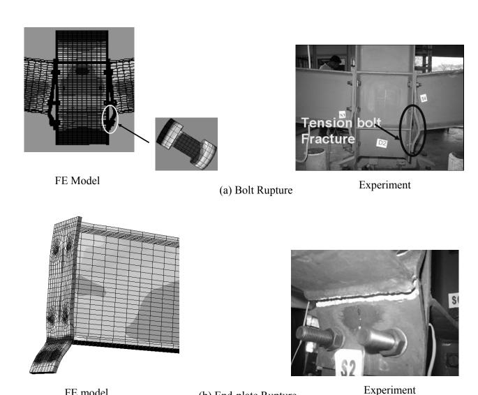
Figure 18. Failure Modes
