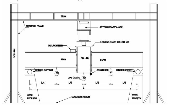
Figure 3. Test Setup and Instrumentation
