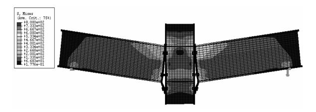
Figure 17. Stress contour at failure
