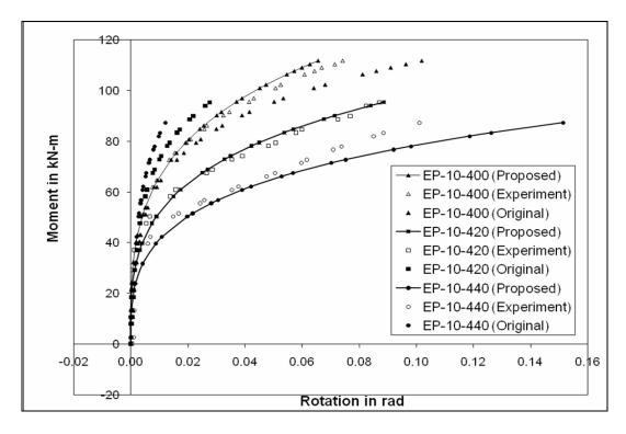
Figure 20. Comparison of M-θ<sub>r</sub> Curves of Proposed Model with Experiment and Original Model for All 10 mm Specimens
