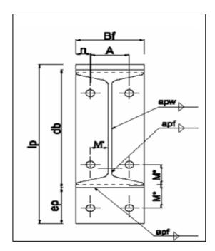
Figure 2. Notations used in the Endplate Connections
