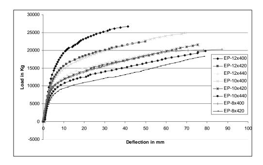
Figure 8. Load-Deflection Behaviour of Different Endplate Specimens
