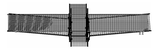
Figure 13. FE Model and the Deformed Configuration of a Typical End-Plate Connected Beam Assembly Model
