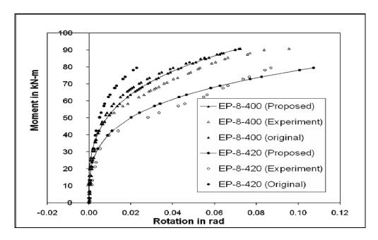
Figure 19. Comparison of M-θ<sub>r</sub> Curves of Proposed Model with Experiment and Original Model for All 8mm Specimens
