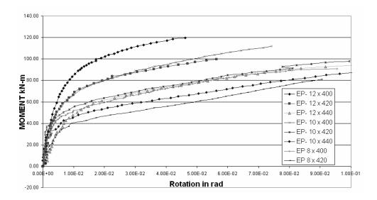
Figure 7. M-θr Relationship of Different Endplate Specimens
