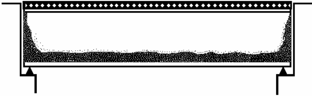
Figure 2(b). Typical Locations where Corrosion can Occur on a Steel Girder Bridge
