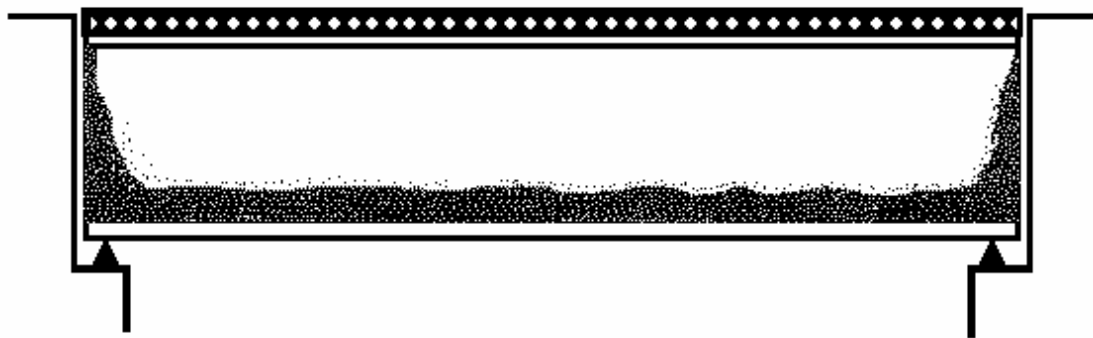
Figure 3(b). Typical Locations where Corrosion can occur on a Steel Girder Bridge
