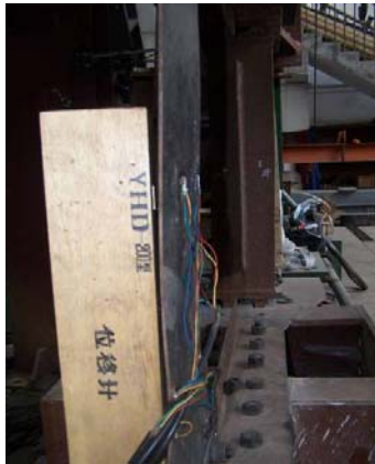
(a) Buckling at the beginning of loading
