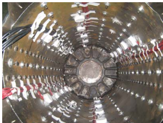
Figure 3. Protection of Pressure Cells and Strain Gauges
